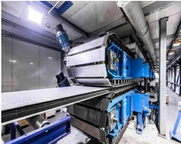
建筑金属夹芯板智能生产线(双履带) Intelligent production line for building metal sandwich panels
